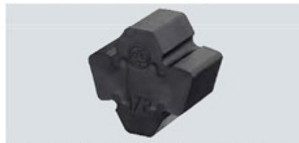
The flexibles of the N-EUPEX DS series are subjected to compression and bending forces. If the flexibles are irreparably damaged, the metal parts turn against one another without contact, and the power transmission is separated. Fitting new flexibles will make the coupling once more usable. The capacity of the N-EUPEX DS series to shed overloads is especially in demand for highly sensitive machines.
