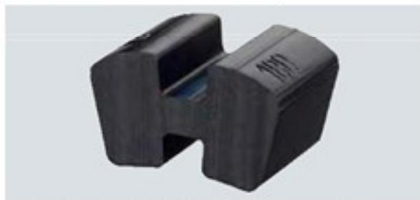
The flexibles of the N-EUPEX coupling are subjected to compression. If the flexibles are irreparably damaged, the hub parts come into contact with metal. This "emergency operation capability" is required, e.g., in the case of fire pump drives.
