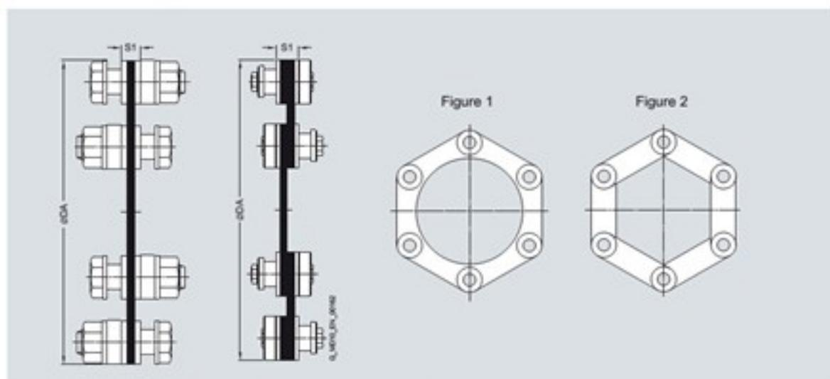
Mainly ring plates (Fig. 1) are used for the plate packs. Sizes 298-6 and 325-6 comprise side-bar plates (Fig. 2).
