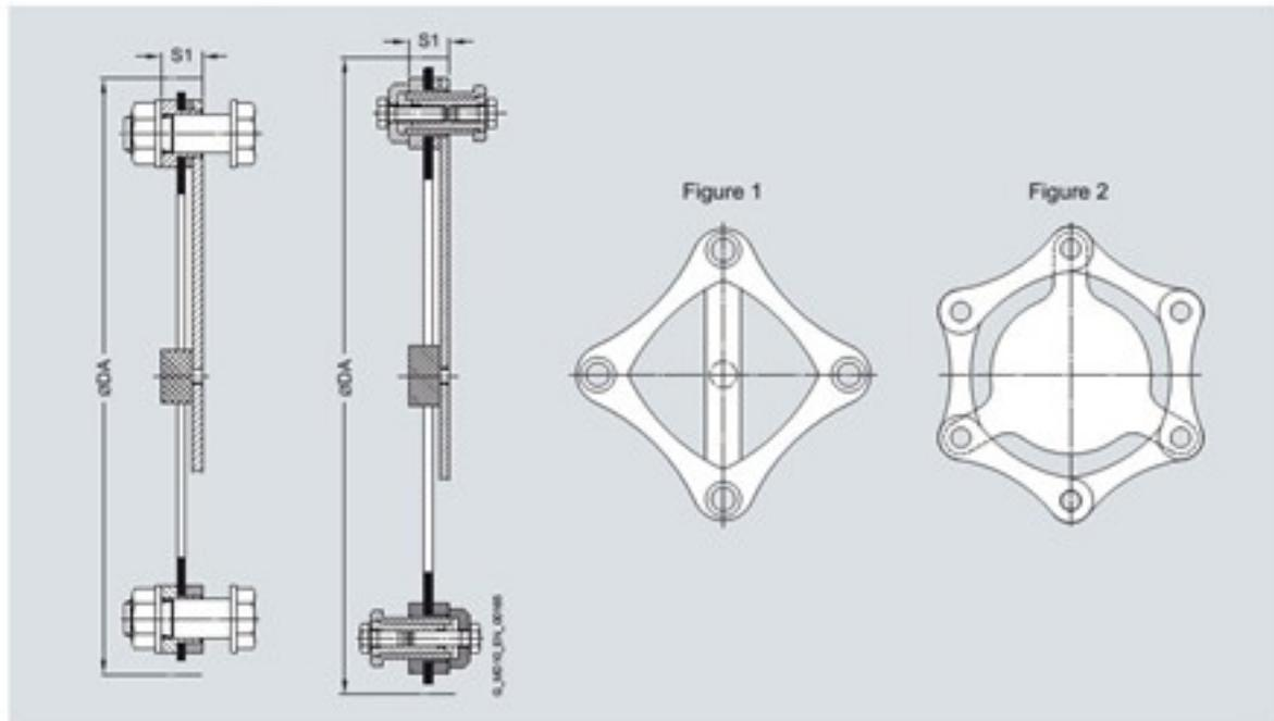
Plate packs of the ARW-4 series comprise ring plates (Fig. 1), those of the ARW-6 series side-bar plates (Fig. 2).
