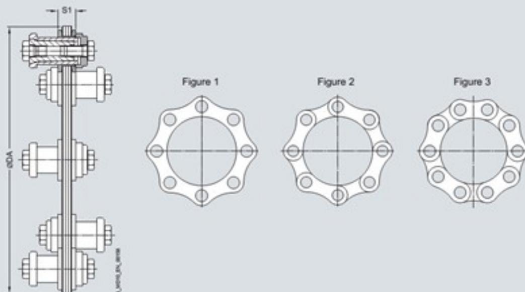
Plate packs of the ARC-8 series up to size 595-8 comprise ring plates (Fig. 1) and from size 630-8 side-bar plates (Fig. 2).
