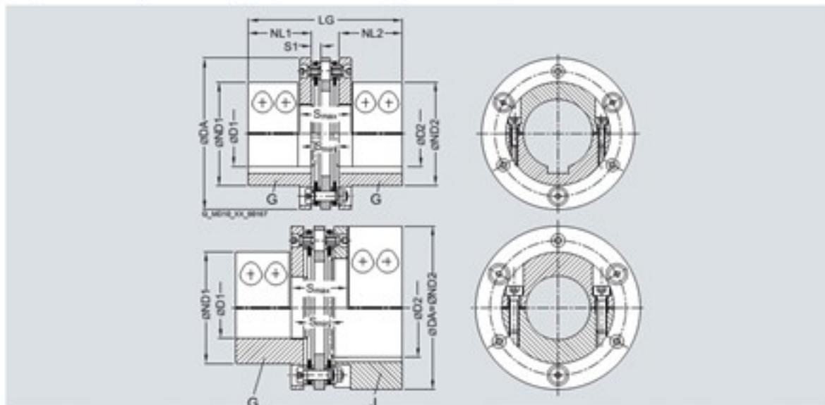
The shaft tolerance must be specified in the order. To specify, -Z must be added to the product code and the order codes Y26 and Y27 with plain text specification of the shaft tolerance for D1 and D2 must be added as well.
